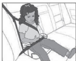
Backless booster with belt-positioning strap
